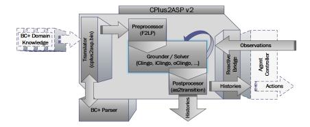
The "reactive bridge" is a new software component, and acts as an intermediary between OCLINGO and a user-provided agent controller system. It allows the agent controller system to provide an  $\mathcal{OBC}$ + observation stream during execution and receive updated solutions in the form of transition system histories.
