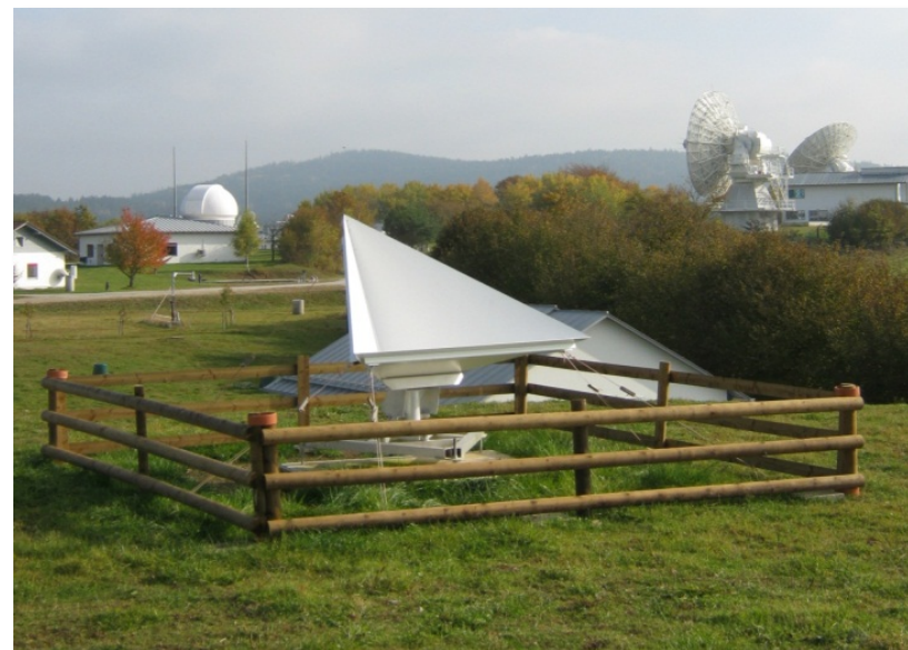
reference corner reflector, Wettzell
