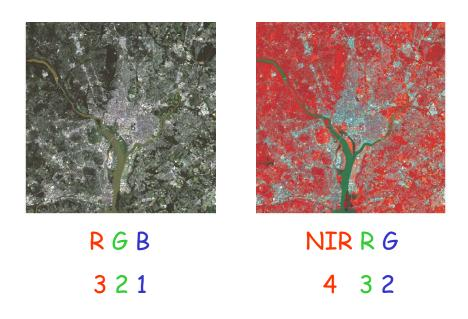
Reflected energy for each pixel in the frequencies Blue, Green, Red & Near Infrared
