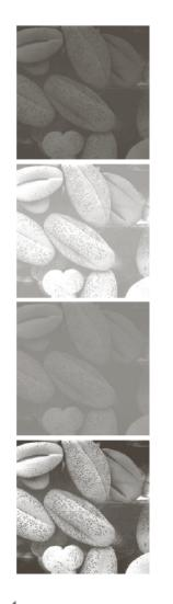
• All 4 images are mapped to a similar output image by applying the same histogram equalization function
