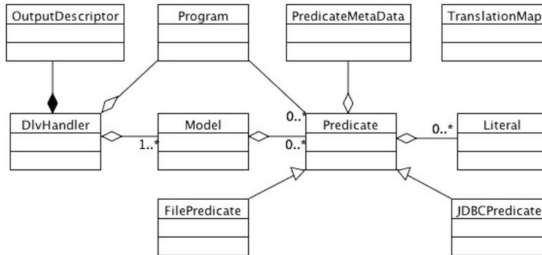
**Fig. 1.** The *DLV* package UML class diagram.
